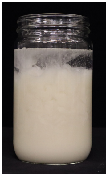
Figure 2: Resicore XL dilution in water without agitation
